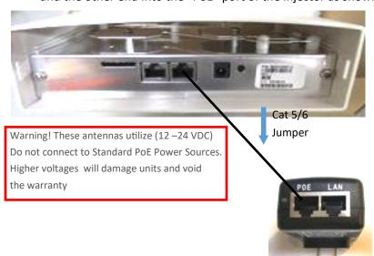
O With another CAT5/6 jumper cable, insert one end into the "LAN" port of the Injector and the other end into a spare data port of your Switch or Router that is Connected to an Internet source as shown at the top of page 2.
